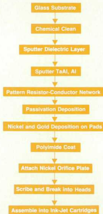
Fig. 3. Flow chart of basic printhead fabrication process.
