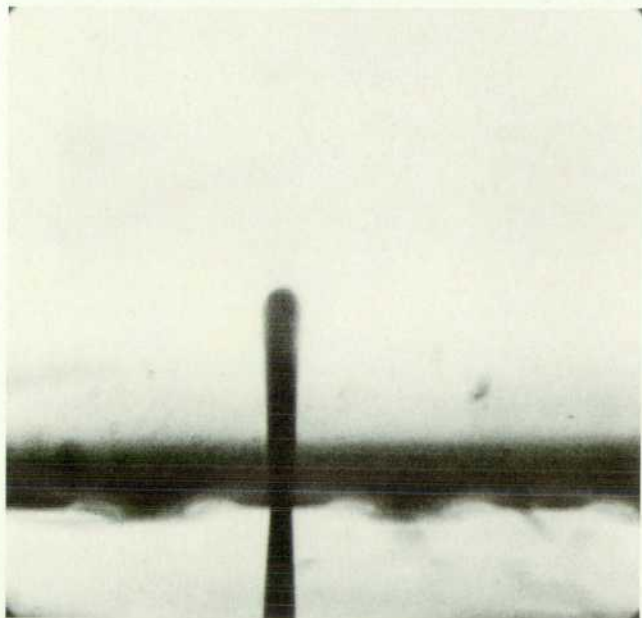
Fig. 8. Photomicrograph of the ejection of an ink droplet 20 \mu\text{s} after the application of the electrical pulse to the heater.
