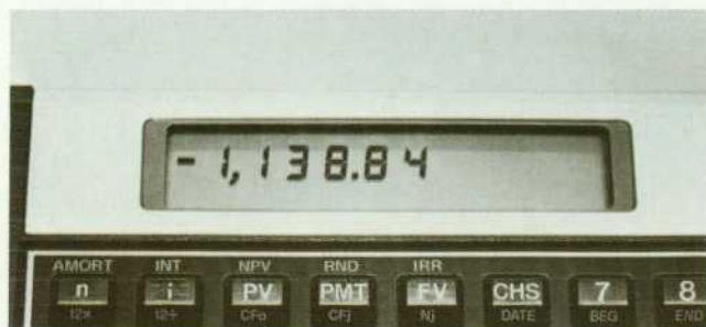
Fig. 3. Top-row-key interface for solving time-value-of-money problems on HP-12C Calculator. On the HP-18C, the top-row-key interface has become a more generalized softkey structure where the key labels are displayed on the bottom of the display above the keys.
