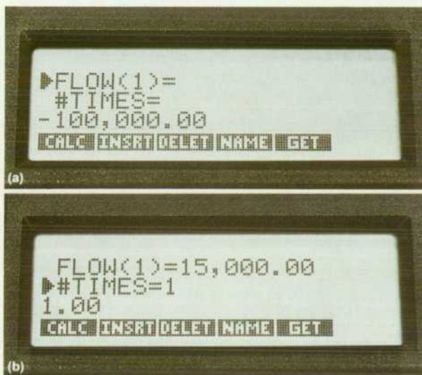
Fig. 1. HP-18C displays for cash flow analysis example. (a) Prompt display for first cash flow entry. (b) After first entry of 15,000 is input, the display prompts for the number of times entry occurs. A value of 1.00 is displayed as a default value. (c) Pressing the INPUT key prompts for the next entry. (d) After completing the cash flow entries, pressing the CALC softkey gives this display. Entering the desired interest value and pressing the 1% key then allows calculation of the net present value, net uniform series, or net future value.
