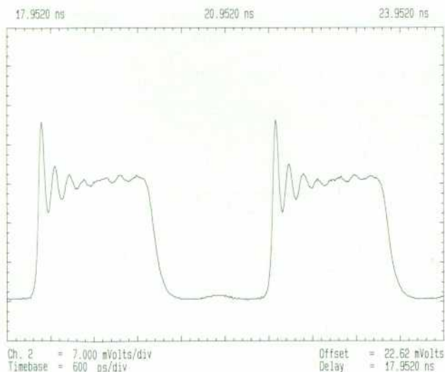
Fig. 1. Typical output waveform of a directly modulated laser.
