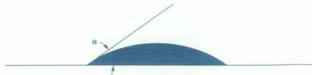
Fig. 2. Solder bead formed by reflowing paste on a plain Cu surface. \alpha is the wetting angle.
