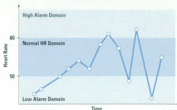
Fig. 2. Heart rate (HR) alarm test principle.
