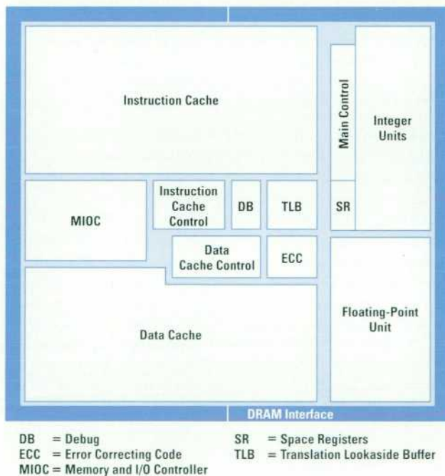
Fig. 3. The final PA 7300LC floor plan.
