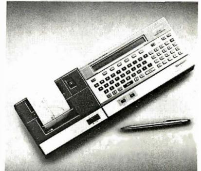
a full upper and lower case ASCII character set, as well as providing user-definable function keys for rapid programming and operation. The optional printer provides four-color graphic capability, nine different character sizes, bi-directional line feed and x,y plotting capability. The printer also incorporates a dual cassette interface for program and data storage/retrieval. Sharp Electronics Corp., 10 Sharp Plaza, Paramus, NJ 07652, (201) 265-5600.
