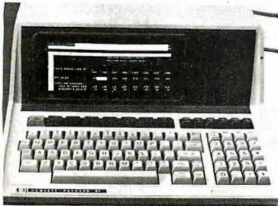
the display. User RAM can be increased to a maximum of 544K bytes with HP memory modules, which come in increments of 32K, 64K, or 128K bytes of RAM. Prices range from \$3,995 to \$7,995. Hewlett-Packard, 1820 Embarcadero Rd., Palo Alto, CA 94303.
