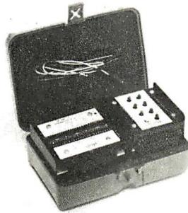
monitored through its current limiting circuitry, to maintain a nominal current drain of 3 mA over a +3 to +25 voltage range. The model 50 Breakout Box provides 24 DIP switches and test points on both sides of the switches to enable reconfiguration of the RS-232 interface. For multiple terminations, it provides common bus points. Price is \$195. Remark Datacom, 4 Sycamore Dr., Woodbury, NY 11797, (516) 367-3806.
