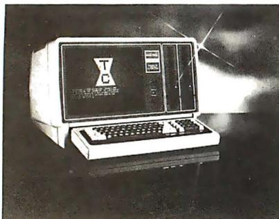
RAM memory storage and 2.5M bytes of disk memory using two built-in, "thin line" double-sided 8-in. disk drives. Additional external disk storage may also be added. The desktop computer will be available in two versions, both with 128K memory.
