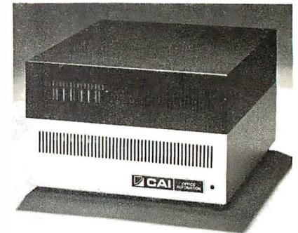
support up to 20 full-time, multi-function work stations. More stations can be added by interconnecting two or more units. A remote option permits the OSI to service clusters of up to seven remote stations on a single modem line. Century Analysis, 114 Center Ave., Pacheco, CA 94553, (415) 680-7800.
