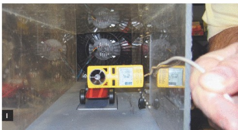
Fig. H: The wind tunnel with air intake (exhaust fan) and straightener. Fig. I: Testing windspeed with a small anemometer.
