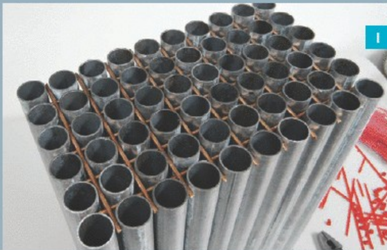
between each tube and the next. After clamping one end, it's easy to insert spacers at the other. Fig. H: The completed, clamped array. Fig. I: Wider spacers (such as
