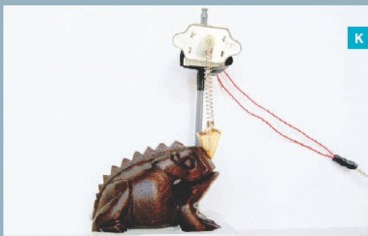
Fig. I: When current is applied to the solenoid, the drumstick is pulled down. Fig. J: MIDI jack pins 4 and 5 transmit data to the Drumbot, pin 3 is for chaining
