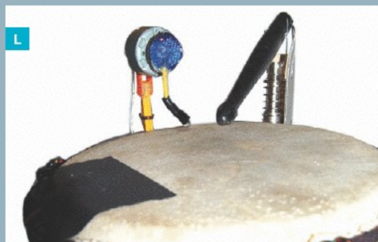
multiple devices. Fig. K: A rotary motor spins a striker to play this woodblock. Fig. L: A solenoid and rotary motor play this drum.
