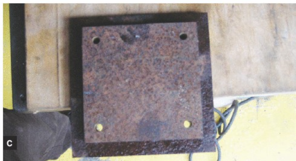
smallest-diameter bit possible. Fig. C: Drill intermediate-sized holes, working up until you get to the size hole you want. It's a perfect match!
