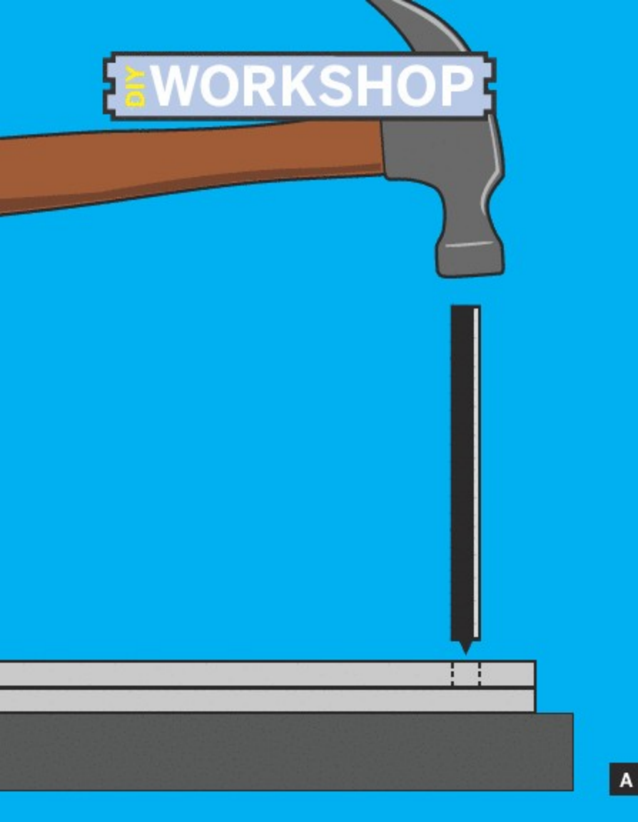
Fig. A: Put a 1/4"-diameter transfer punch down each hole you are duplicating, and tap with a hammer. Fig. B: Before using the desired-size drill bit, minimize wandering by making a preliminary pilot hole using the
