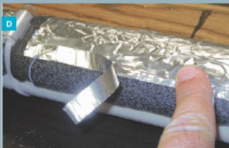
Fig. C: The right end of the pipe, with the tuning peg for tightening the string. Fig. D: Taping stripped wire to the foil drum pad.
