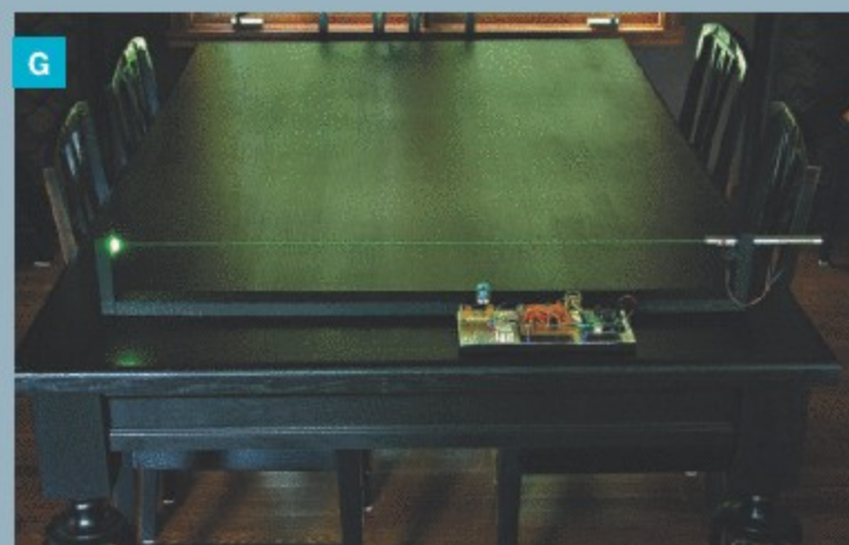
reflective laser pointer barrel. Fig. F: The power supply board, detector board, and Arduino on a wooden base. Fig. G: A 1-string optical theremin with green laser.
