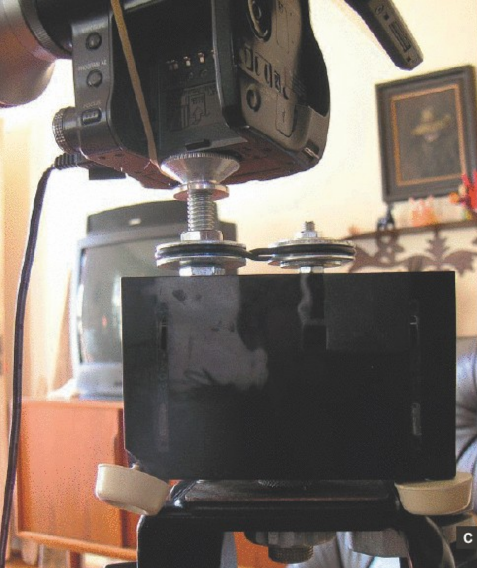
Fig. C: The two-shaft clock mount carrying a camcorder, with the belt reversed for counterclockwise motion. Fig. D: The two-shaft clock mount with the belt in the clockwise configuration. Fig. E: Meade Autostar
